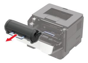
**3** Remove the used imaging unit.
