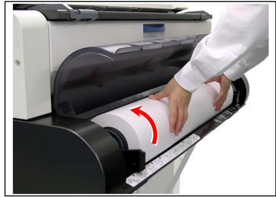
8. Rotate the roll media in the arrow direction and insert the leading edge of the roll media to the media path until it touches the feeding rollers (4).
