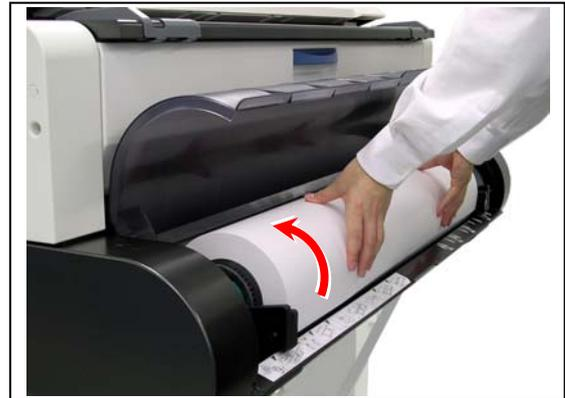
2. Rotate the roll media in the arrow direction and insert the leading edge of the roll media to the media path until it touches the feeding rollers (1).
