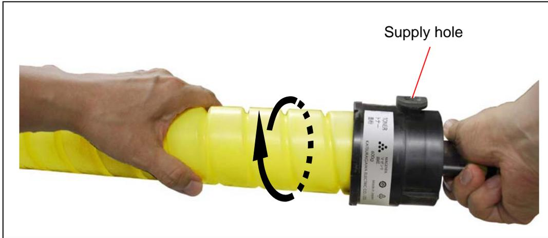
5. Keeping the Supply Hole upward, insert the Toner Cartridge to the corresponding color slot until it stops.
