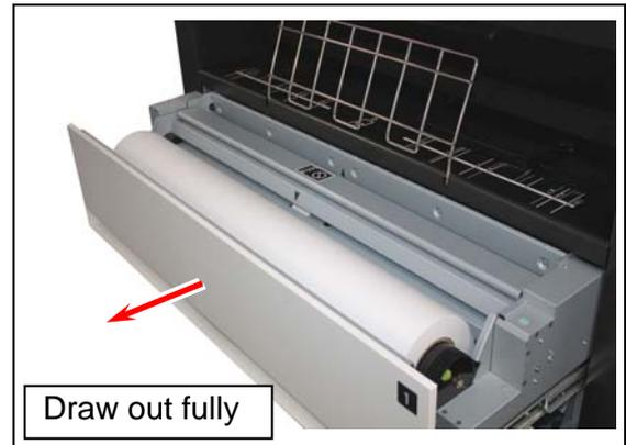
6-3. Insert the leading edge between the feeding rollers. It will automatically go into the roll media's standby position. (Auto Media Loading)
