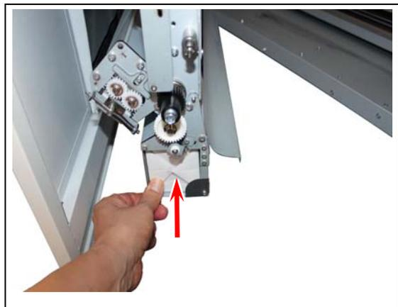
8. With pressing, turn the stopper to the arrow direction to release the Waste Toner Box. Keep it pressing even after releasing.
