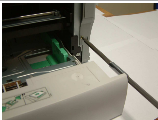
Front mounting screw of the right hand side cover
