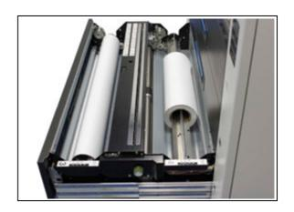
5. Insert the leading edge of media under the feeding roller.
