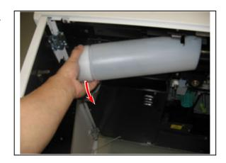
5. Shake the new Toner Cartridge fully to loosen the toner.
