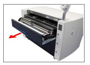
2. Retrieve the Roll Spool to the arrow direction a little to disengage the gears on the left, and remove the Roll Spool from the deck.
